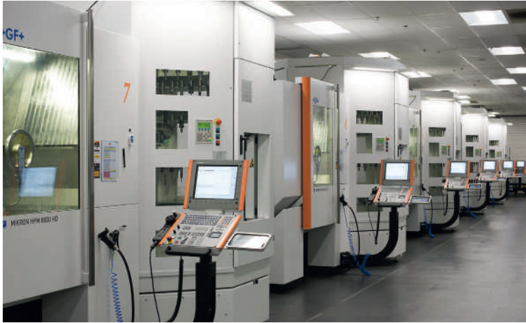
TRD runs eight GF machines in total: in a fully automated production cell, engine blocks, cylinder heads, pistons, and other engine components are milled by 5-axis machining centers.
