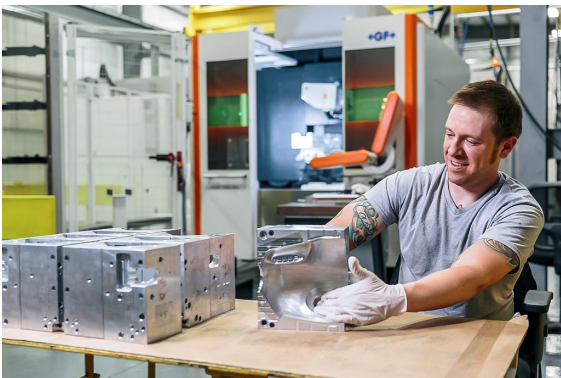
Every year, Custom Etch engraves between 3’000 and 4’000 individual molds for the production of PET bottles.
