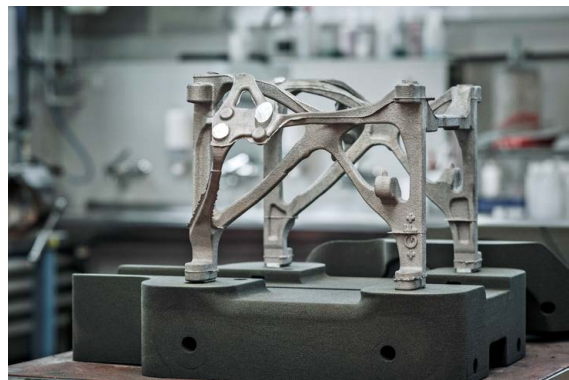
The two aluminum axle carriers hold the front and rear axles of the pod chassis and provide stability. They are both 35 cm high, 30 cm wide and 55 centimeters long, and weigh just five and a half kilograms each.
