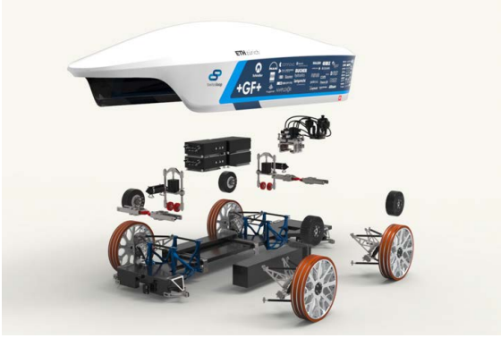
Swissloop's 2018 pod is propelled by four electric motors with an output of 540 hp and can reach speeds of up to 500 km/h.
